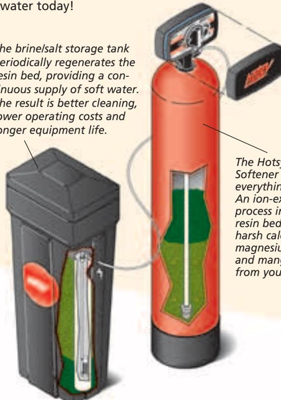
*The Hotsy Water Softener provides everything you need. An ion-exchange process in the cation resin bed removes harsh calcium, magnesium, iron and manganese ions from your water supply.*
